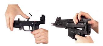
As shown in the figure, first press the recoil spring plate on the upper receiver and at the same time push the lower receiver upwards to close the upper receiver. Then lock the upper receiver by placing the fixing pin in its position before it was opened.
